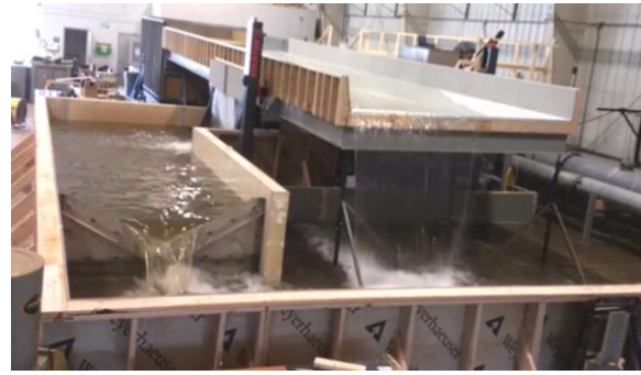
Figure 2. Constructed full-scale test deck during flow testing at IIHR's hydraulics laboratory.
